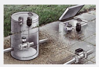
With the MAG 8000 range, it is easy to install a reliable water meter in virtually any environment, whilst maintaining full accuracy, performance and economy of operation.
